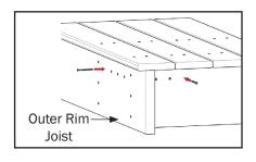
**Step 4:** Measure and mark holes for the Post Mount, specific to your post size. Use 7/16" drill bit with a shank at least 5.5" long. Keep power drill straight while drilling.
