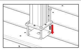
**Step 6:** Place the Under Deck Bracket over the bolt ends, parrallel to outer rim joist as shown, and fasten using a standard washer followed by a hex nut.
