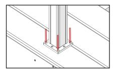
**Step 5:** Place leveling plate between post and mounting surface. Using 3/16" Allen wrench, turn set screws to level post. Use 3/8" x 5.5" Hex Head Bolts to fasten post to decking.
