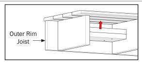
**Step 3:** Fasten each side using three wood deck screws on the bottom board, use four screws on the lower board for the front.
