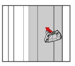
Place Lens sub-assembly over access hole utilizing the adhesive to hold it in place
