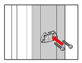
Fasten Lens sub-assembly using #8 x 1" Pan head Screws (*provided*) take care not to overtighten
