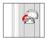
Snap Powder Coated Aluminum Cap onto Lens sub-assembly
