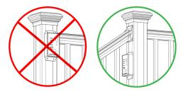
Do not install Control Hub in direct view/close proximity of post cap lighting, as it will cause undesired results.
