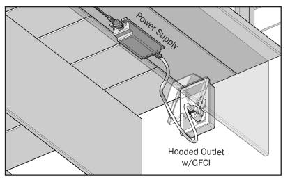
The Power Supply can be mounted under the deck, and out of sight. Supplied input wire with plug must be connected to a receptacle protected by a GFCI feature with a hooded cover. If no GFCI is available, a licensed electrician must install one. Do not use an extension cord.
